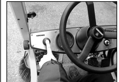
Switch hazard warning lights on / off.
